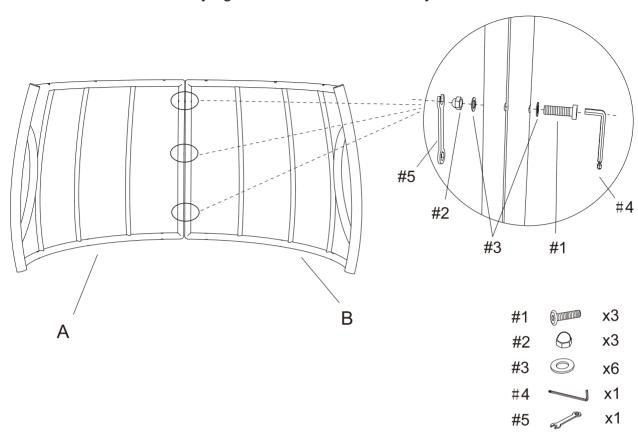
Step 2. Attach bottom panel (part D) to panels (parts A & B) using bolts (part #1), flat washers (part #3), nuts (part #2), allen wrench (part #4) and wrench (part #5).
