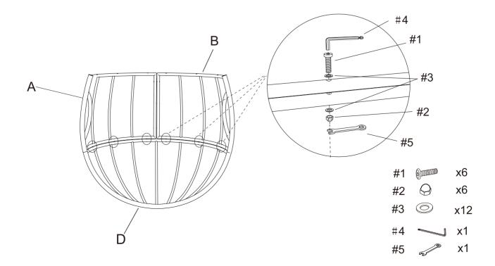
Step 3. Attach top panel (part C) to panels (parts A & B) using bolts (part #1), flat washers (part #3), nuts (part #2), allen wrench (part #4) and wrench (part #5).
